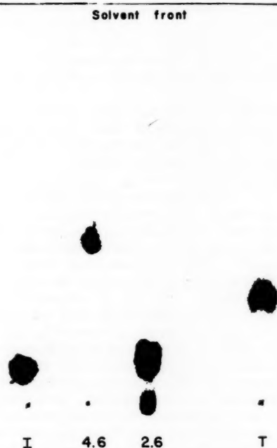
FIG. 5. Paper chromatogram of concentrated ether extracts of field grown tomato plants not treated with tryptophan. Chromatogram developed with isopropyl alcohol, concentrated ammonium hydroxide, water (80:10:10, v/v) and sprayed with Ehrlich's reagent. The numbers refer to the extraction pH. I is synthetic indoleacetylaspartic acid and T is a tryptophan marker. Extracts from approximately 100 gm fresh weight of tissue were applied to the chromatogram. The substance extracted at pH 2.6 ( R_f 0.11) yielded tryptophan on hydrolysis.
